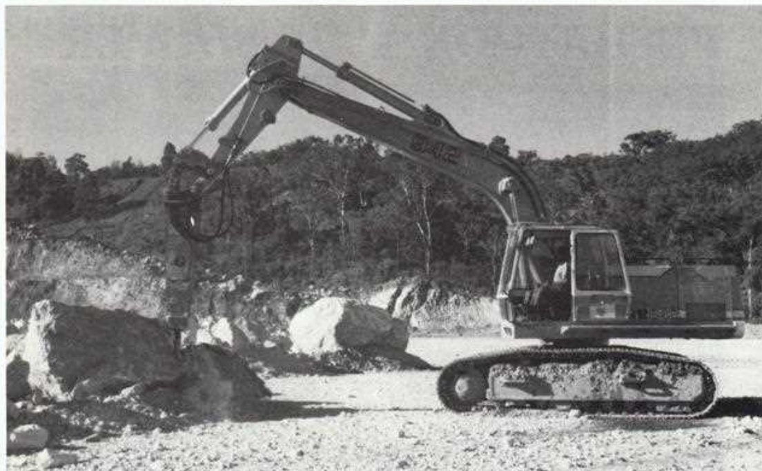
● Proof of the pudding - the rock breaker made short work of this massive hunk of rock.
