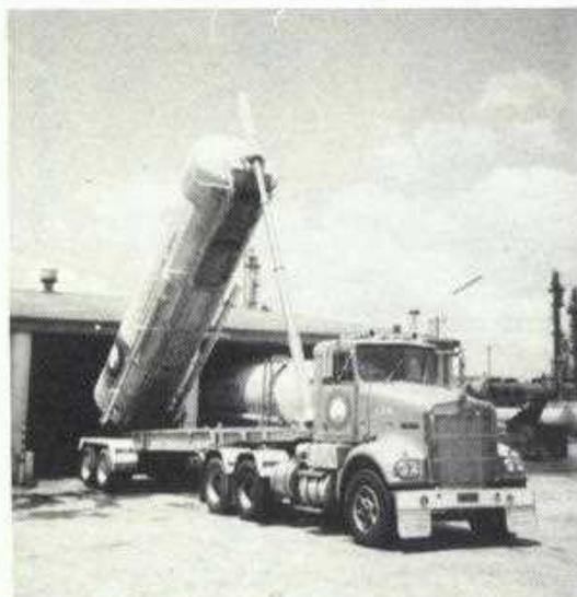
Unit 135 (pictured) is a W925 SAR Kenworth prime mover, powered by a Formula 290 Cummins engine, driving through an RTO 9509B Road Ranger transmission to SSHD 44,000 lb capacity Rockwell differentials, with a ratio of 5.29 to 1, giving it a possible top speed of 103 KPH.
