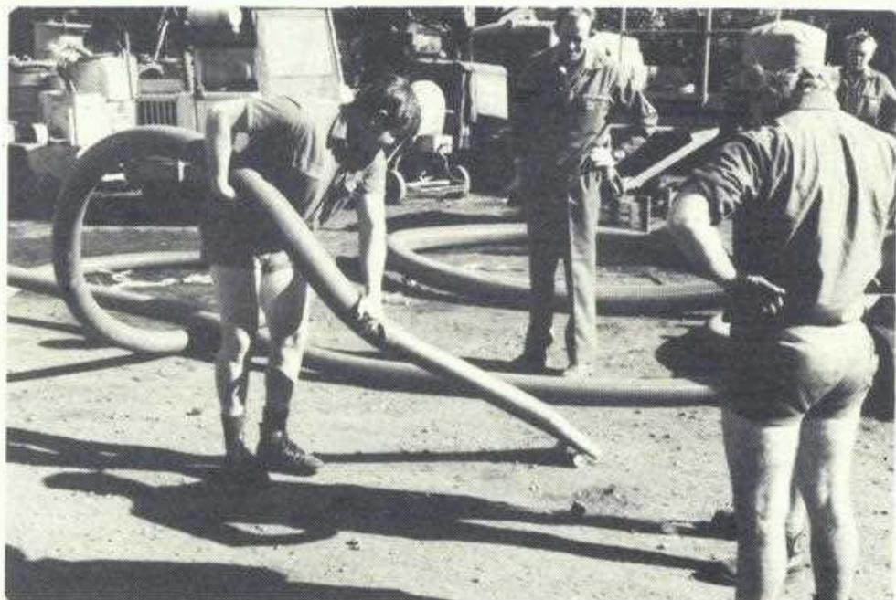
*An outdoor demonstration of the use of the flexible hose. This RENVAC Vacuum Loader was specially equipped with wheels to give it ready mobility at Berrima.*
