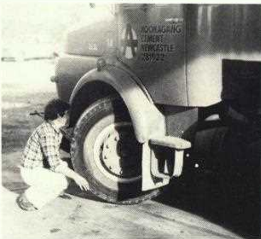
♦ Allan Baker, transport mechanic, does a brake check on one of the Mercedes prime movers.
