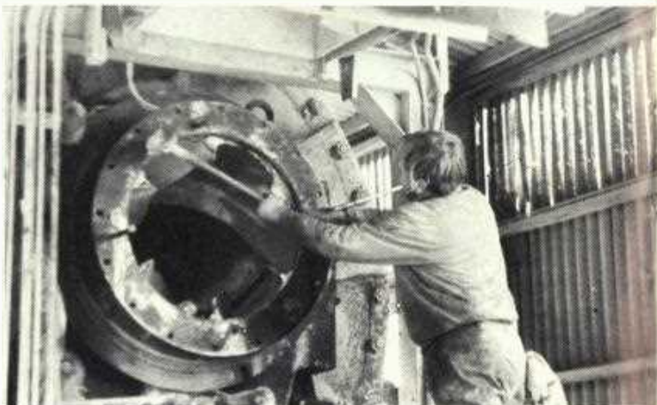
PAUL Harris, maintenance fitter, needed his 14lb persuader to draw out the original feed end trunnion liner from the ball mill for replacement.
