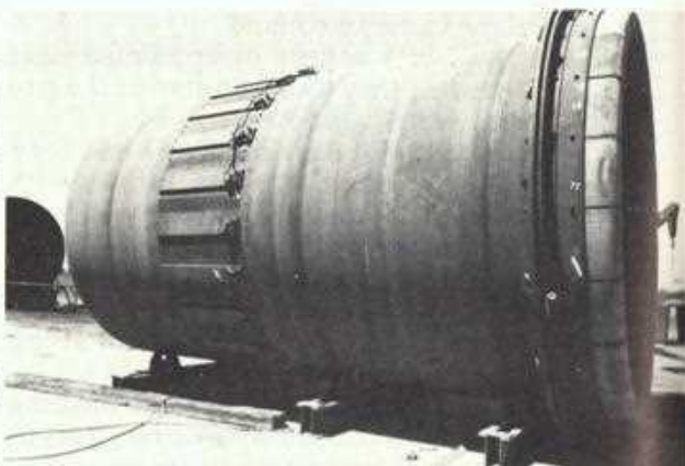
Top left: The two new sections for the kiln. Above: The firing end of kiln to be replaced. The picture shows the tracks set for removal of the section and support legs under the remaining section. Below left: The new section of the kiln ready to fit into place at No. 2 tyre station. Below: A close up of new firing end section.
