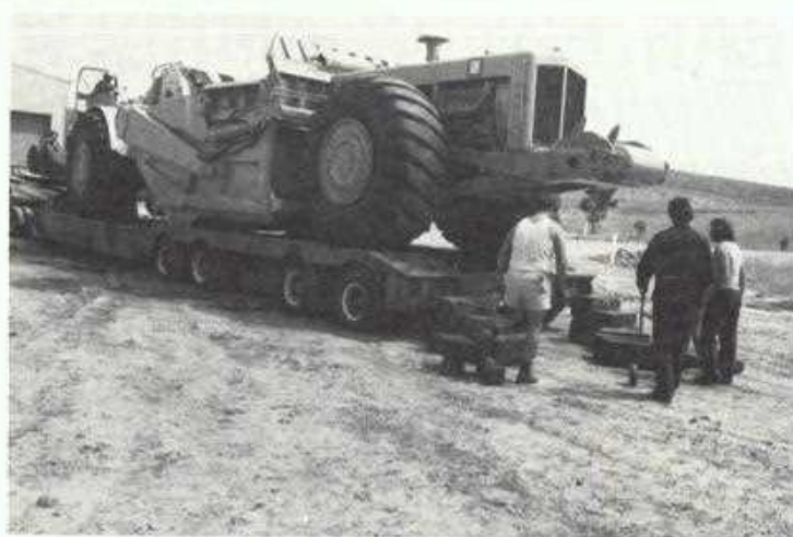
The new Terex twin power scraper arrives at the Waurm Ponds quarry. The scraper powered by two 8V 71 Series GM diesel engines is being unloaded by L to R — G. Carey (in driver's seat), Semi-driver; D. Love and G. Sharp.
