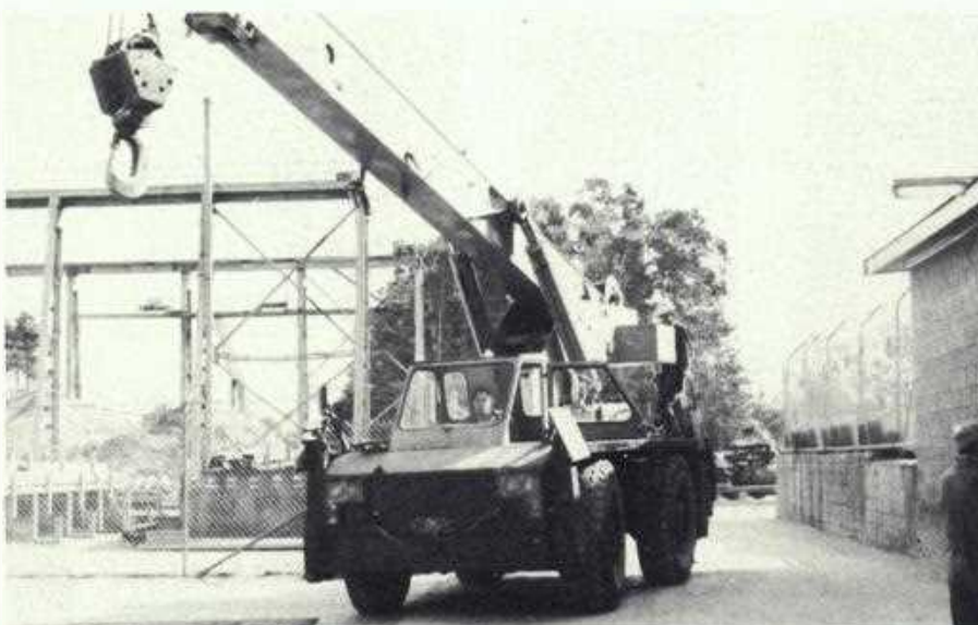
Berrima's mobile muscle, Cole's "Hydra Husky Crane". This machine is one of the Maintenance Department's most useful tools and can lift 12 tonnes with its 60' hydraulic jib. The crew here are driver, Bill Hutchings and crane chaser, John Steward.
