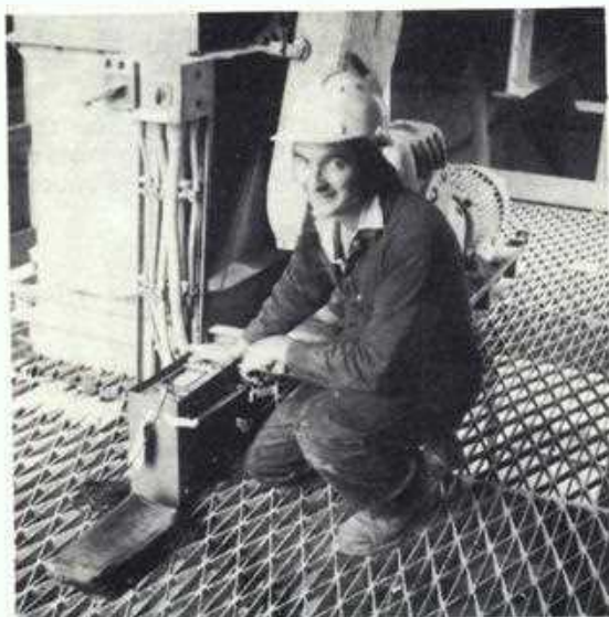
Berrima Maintenance Dept.'s Inspector, Mick Baker, using the "Mepa" 10 bearing test meter.
