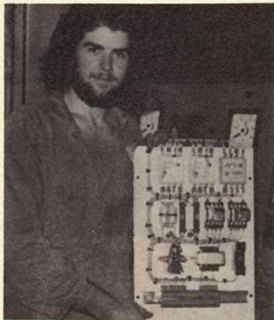
Above: Dennis Harrold with a control panel he has made, using solid state logic modules for the first time at SPC. These replace electro-mechanical relays presently used at Berrima.
