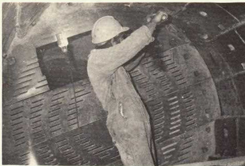
Above:— Fourth year apprentice Mick Eirth removes one of the many steel liner plates during a recent overhaul. In the background can be seen the perforated diaphragm used for separating the Cylpebs and steel balls.
