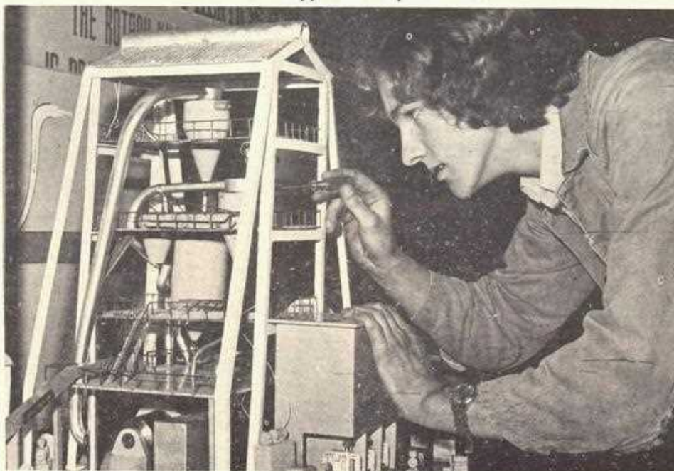
SPC Apprentice Gary Hinton assembling the model of No. 5 Cement Kiln. The actual kiln is situated at Berrima Plant. It is 560 feet long and 15 feet 3 inches in circumference. It has a capacity output of 1,400 tons of cement clinker per day.
