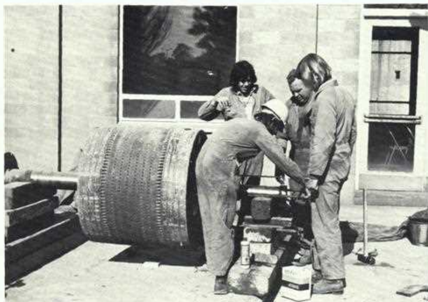
Tradesmen A. Ducks-bury and C. Bloomfield with apprentices D. Harrold and P. Shanks, removing Slip Rings from No. 2 Cement Mill Motor.
