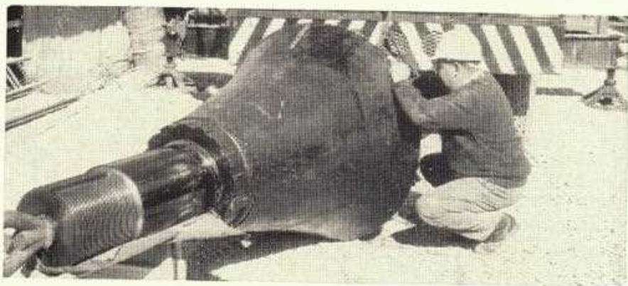
Marulan Fitter, Mick Cosgrove, making an adjustment to the new Gyratory Crusher at the quarry
