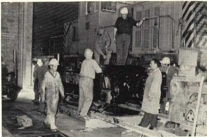
The Maintenance section at Berrima recently changed the bogey of the loco with a new one, which has a much better braking system than the original. Picture shows Foreman Keith Graham supervising the work.
