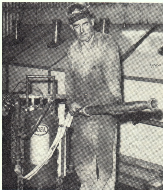
Pictured above is a foam generating fire fighting unit recently installed at the Works.
